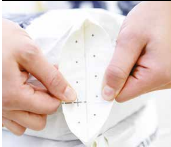
Ultrasonic sealing tightly closes the sack
