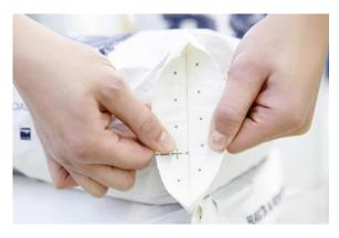
The ultrasonic sealing of the valve results in absolutely tightly sealed and clean paper sacks and optimises the filling process. Copyright: Haver & Boecker
