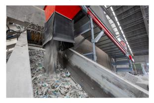
Figure 3. The used paper sacks are shredded and thoroughly cleaned in the unique cleaning plant.
