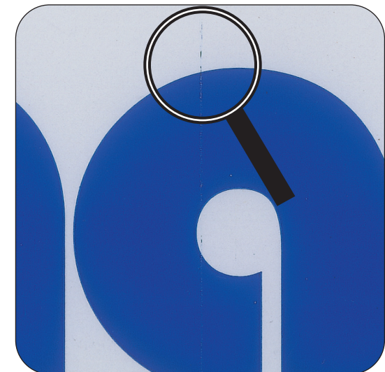
EXAMPLE FOR STREAKING
