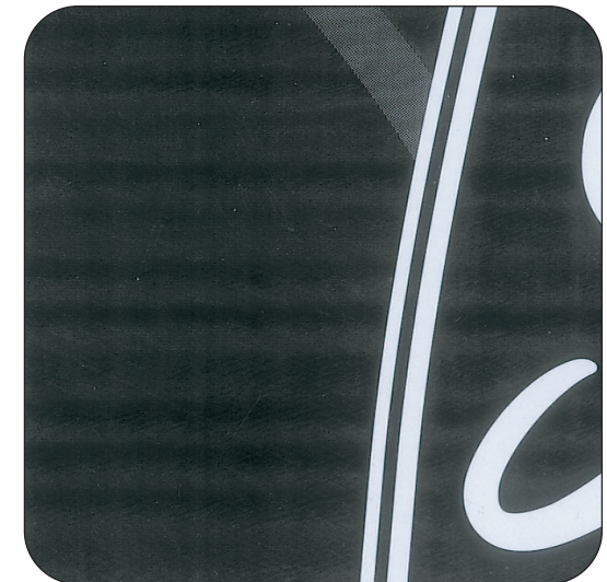
EXAMPLE FOR GEAR MARKS
