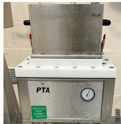
The Somerville Fractionator houses the coarse or fine screen to facilitate separation of fibres from rejects. The fibres are made into hand sheets to assess the properties of the paper.
